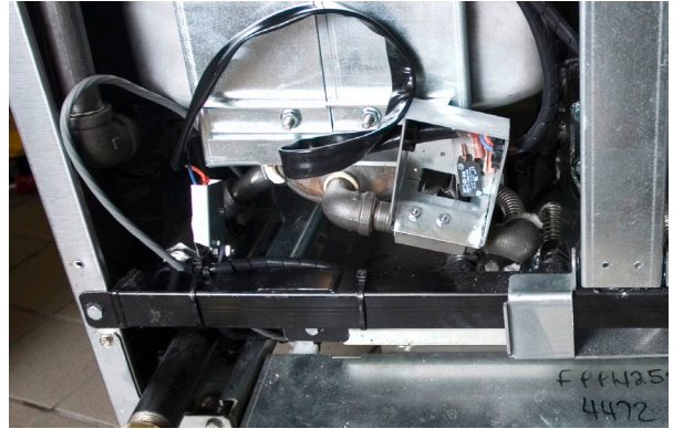
Figure 5 The rear valve switch is shown in place. It is wired in parallel with the existing switch, using piggyback terminals.
