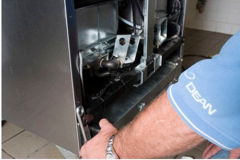
Figure 4 Pry on the loosened manifold as necessary to install the inward pointing elbow.
